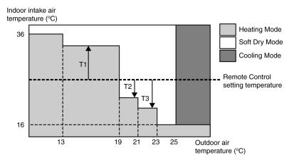
• Every 180 minutes, the indoor and outdoor temperature is judge. Based on remote control setting temperature, the value of T1 will increase up to 10°C, T2 will decrease by 3°C and T3 will decrease up to 8°C.
