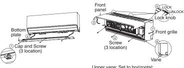
Upper vane: Set to horizontal; Lower vane: Set to slightly below horizontal
