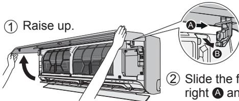
② Slide the front panel to right **A** and pull out **B**.
