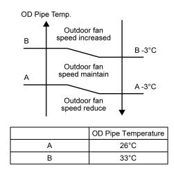
• During above condition, when indoor heat exchanger temperature is below 5°C, the outdoor fan will stop according to outdoor piping temperature as following:
