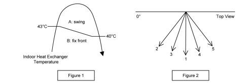
• Manual horizontal airflow direction can be set using remote control; the angles of the vane are as stated below and the positions of the vane are as Figure 2 above.
