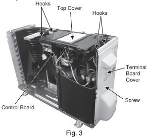
5 Remove the Control Board as follows:
