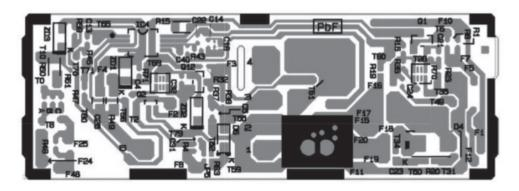
11.1.4 Wireless LAN Module Printed Circuit Board (Network Adapter)
