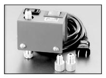
7. HFC refrigerant\_Electric gas leakage tester R32 refrigerant is often used for other mixed refrigerant (R410A, R404A, R407C etc.). Therefore, the usage of existing HFC detectors is possible, but in order to detect more accurately, we recommend to use detectors specially set and adjusted for R32 detection.
