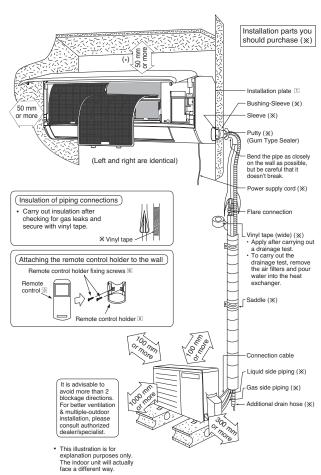
(\*) If holder at the rear of chassis (Refer column "12.2.3 Indoor Unit Installation") need to be used to prop up the unit, this distance shall be 65 mm or more.
