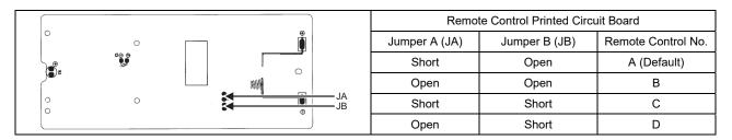
During Remote Control Number Switch Mode, press any button at remote control to transmit and store the transmission code to the EEPROM.
